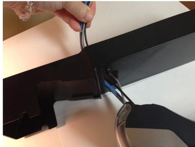
Push cables thru hole and reattach to terminal - Step 4
