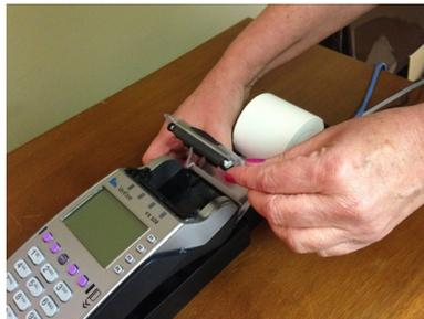
Feed paper into terminal and snap spindle into base - Step 8
