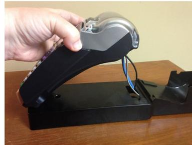
Attaching to base. Hold at angle and press front down then back- Step 5
